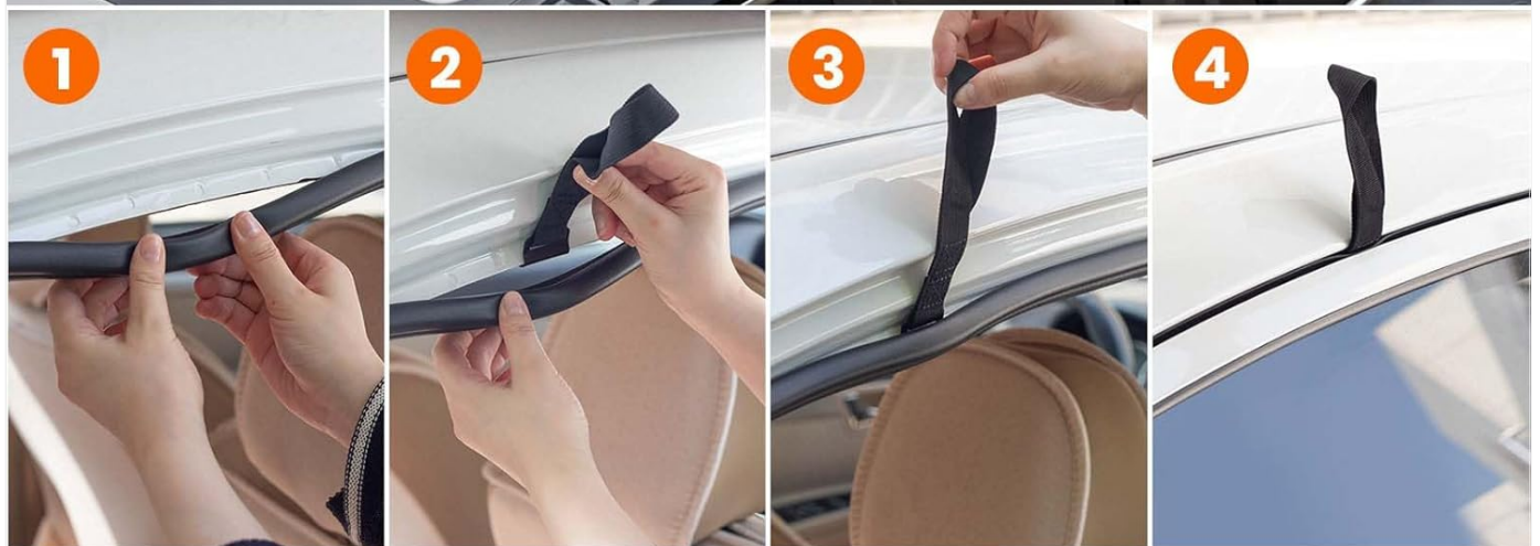
Figure 4: Step-by-step guide for securing the roof bag using the provided door hooks, ideal for vehicles without existing roof racks.
