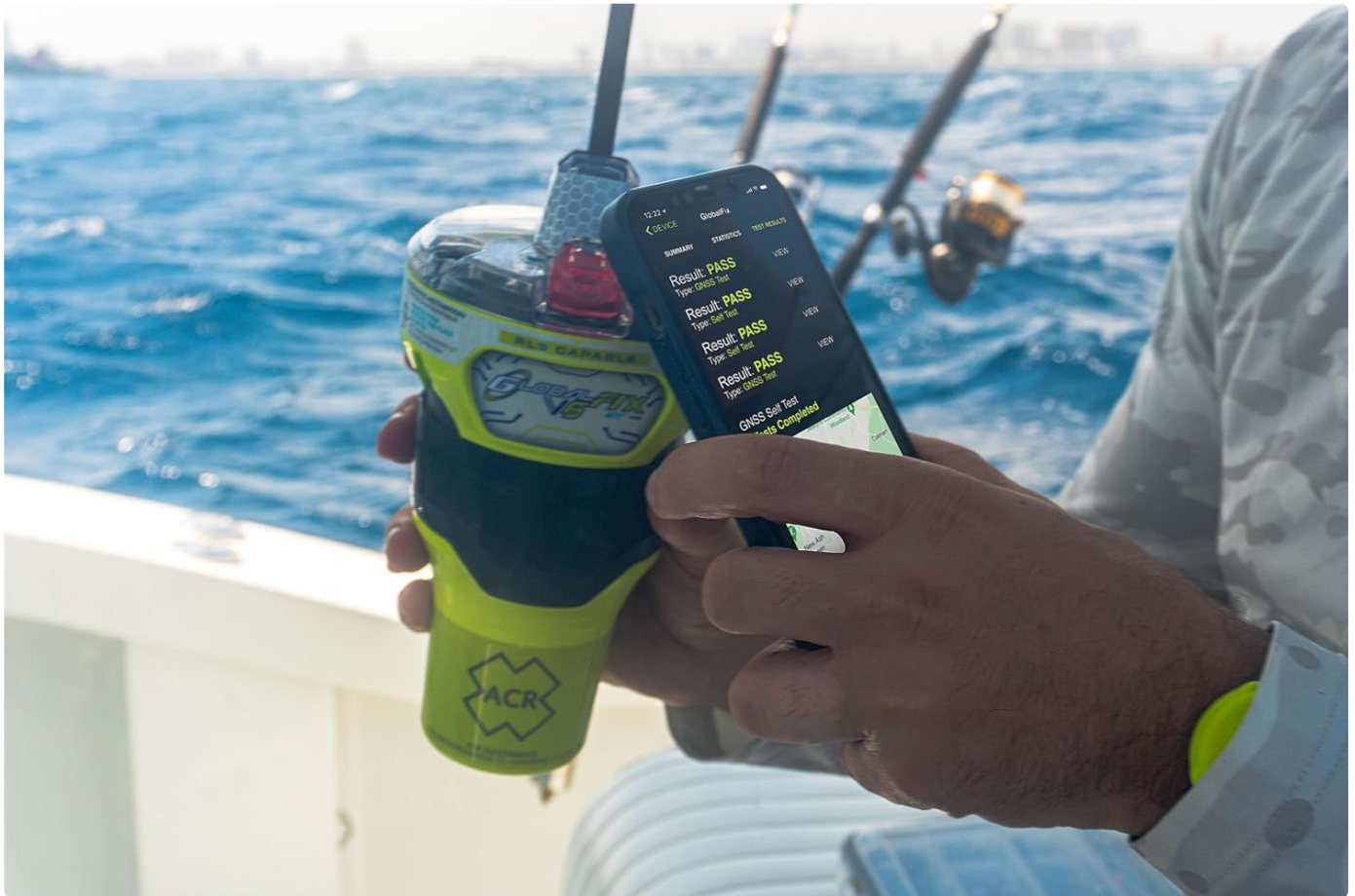
Figure 3: A user interacting with the ACR mobile app on a smartphone, connected to the GlobalFix V6 EPIRB via NFC for diagnostics.
