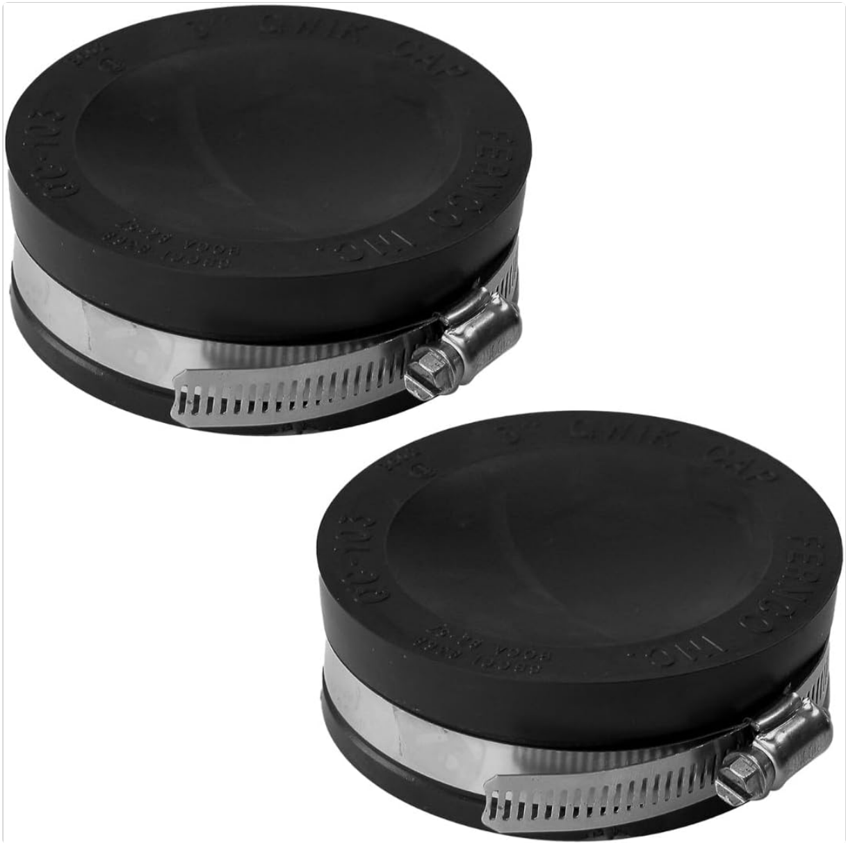
Figure 1: Two Fernco QC-103 Qwik Caps. Each cap is black, made of flexible PVC, and secured with a stainless steel clamp.
