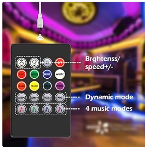
Image: Close-up of the IR remote control, detailing buttons for power, color selection, brightness/speed adjustment, dynamic modes, and music modes.
