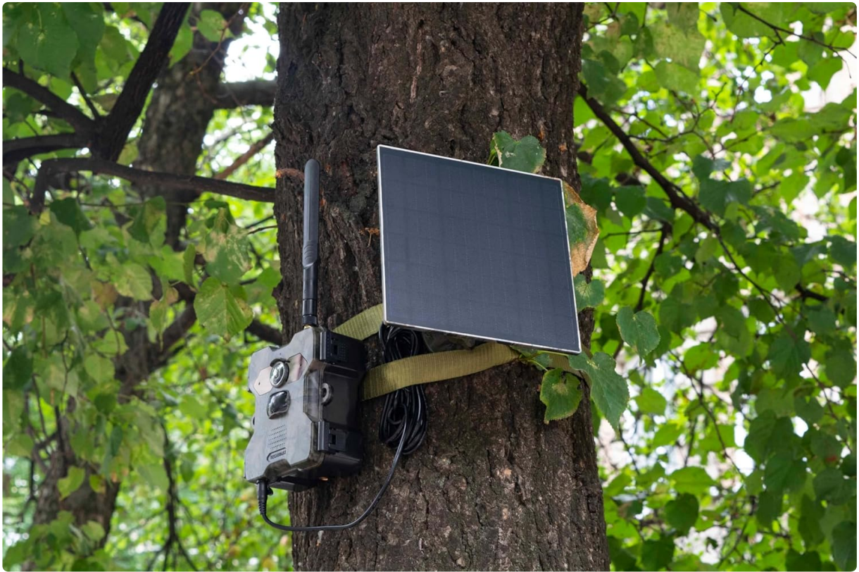
Image: The camera and its accompanying solar panel mounted together on a tree, connected by a cable.
