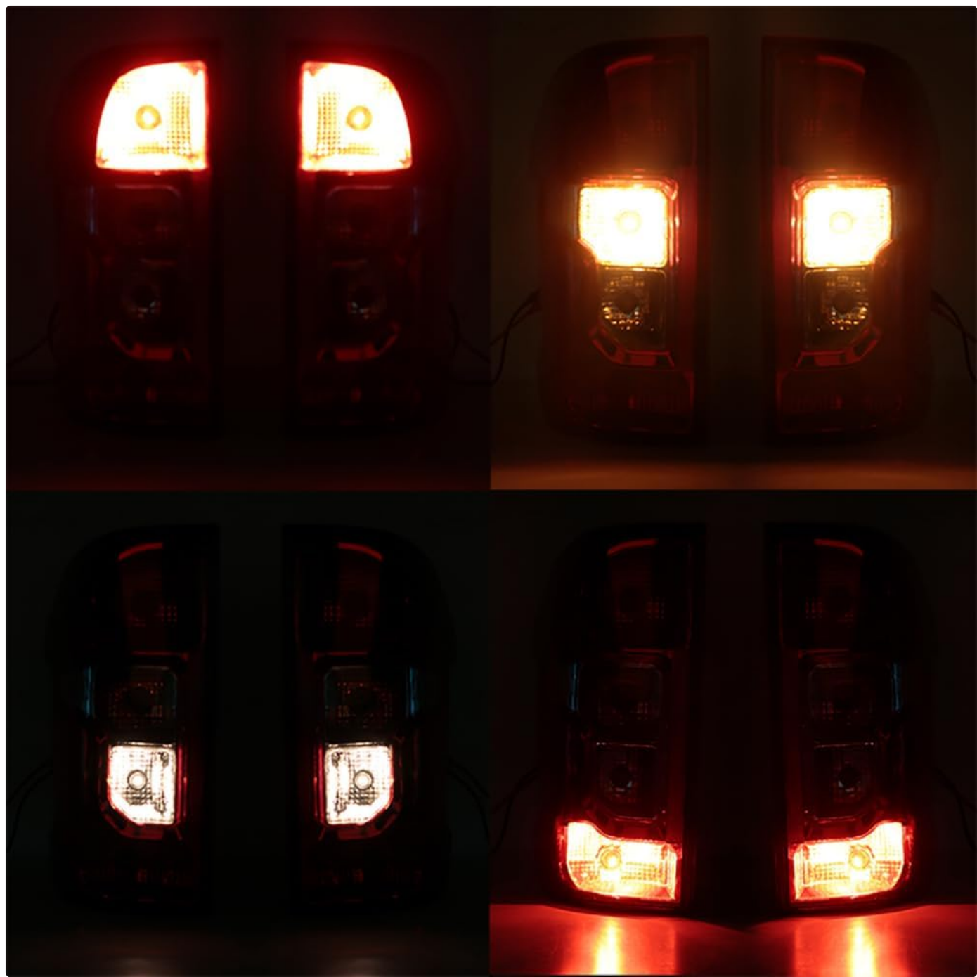
This composite image shows the tail lights in different operational modes: turn signal (top left/right), brake light (bottom left), and running light (bottom right), demonstrating their illumination patterns.
