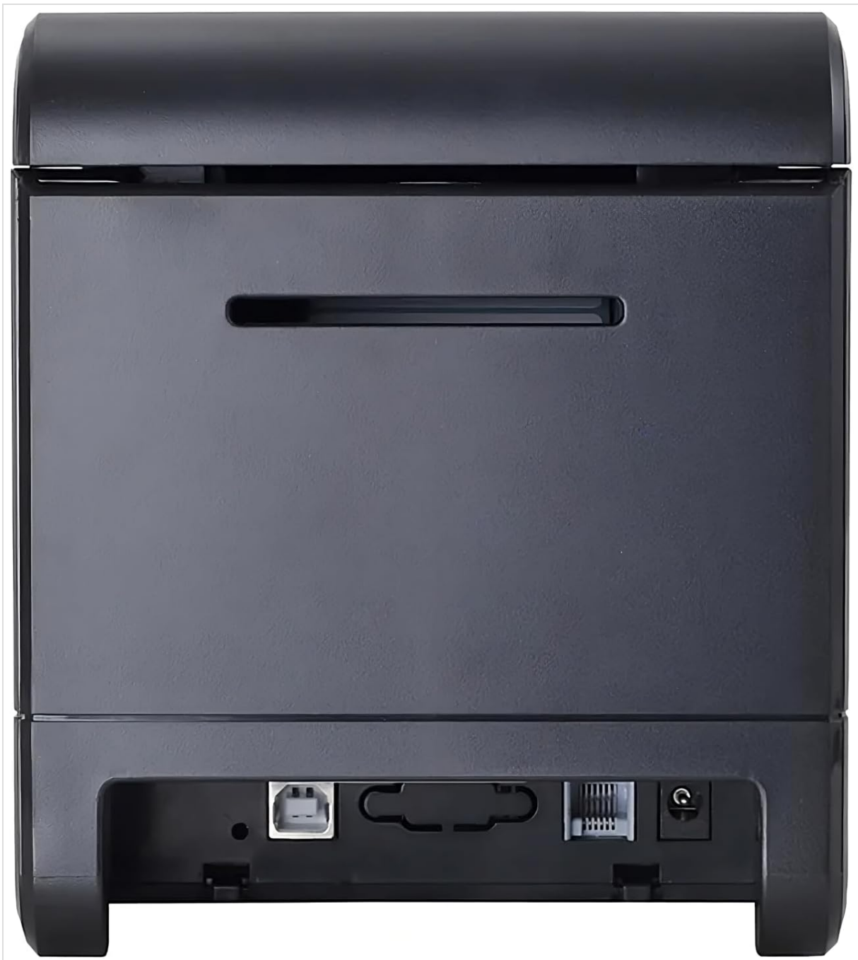
Figure 4.2: Rear view of the Xprinter XP-233B, highlighting the USB, Ethernet, and power input ports.
