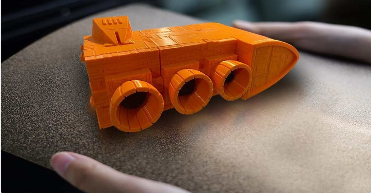
Figure 8: Removable magnetic PEI steel platform for easy print removal.
