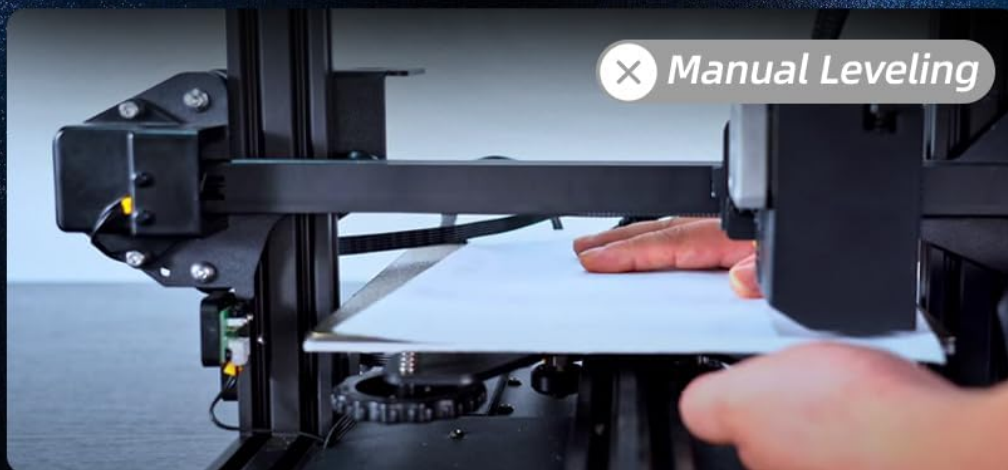
Figure 4: Comparison of 25-point auto-leveling and manual leveling.
