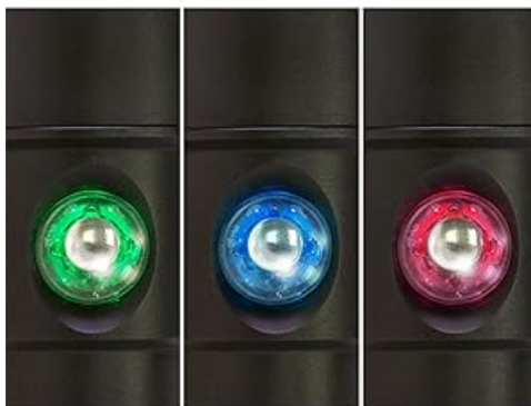
Image: Close-up of the Bigblue VTL 2900's power button, showing its function as a battery level indicator with different colored lights.
