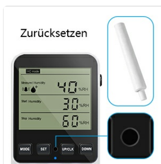
Image: A close-up showing the location of the reset button on the side of the KETOTEK controller.
