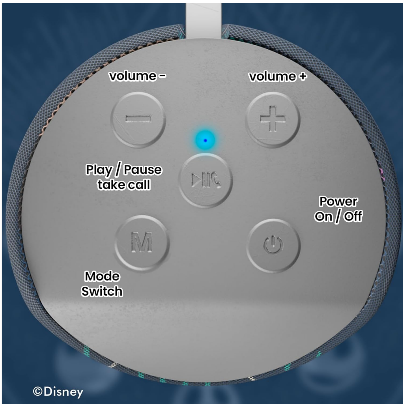
Image: Top view of the speaker showing the control buttons: Volume -, Volume +, Play/Pause/Take Call, Mode Switch, and Power On/Off.
