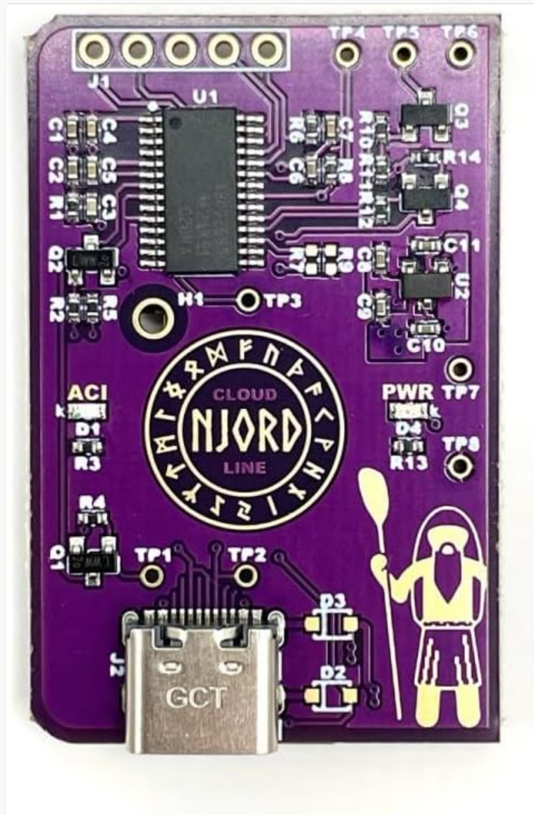
Figure 2.2: Top-down view of the Njord Control Board, highlighting the "Njord Cloudline" branding and component layout.
