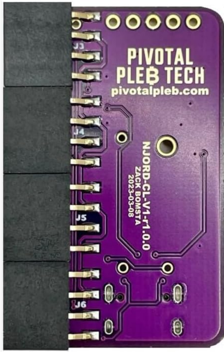
Figure 2.3: Bottom view of the Njord Control Board, showing the "Pivotal Pleb Tech" manufacturer details and model information.
