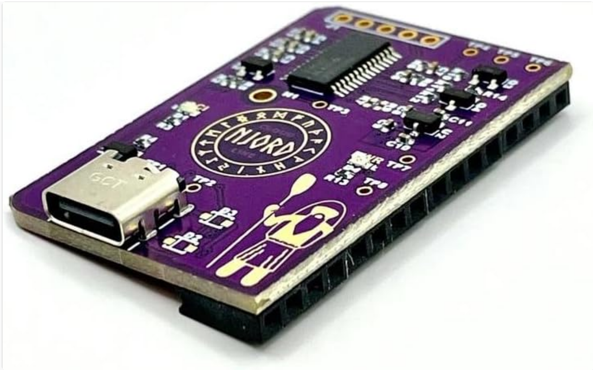
Figure 2.1: Front view of the ALTAIR TECHNOLOGY Njord Inline Fan Control Board, showcasing its compact design and USB-C port.
