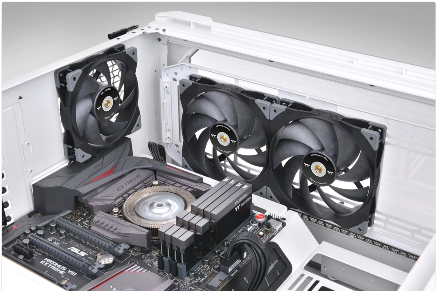
Image: Two Thermaltake SWAFAN GT14 fans installed as exhaust in a PC case.
