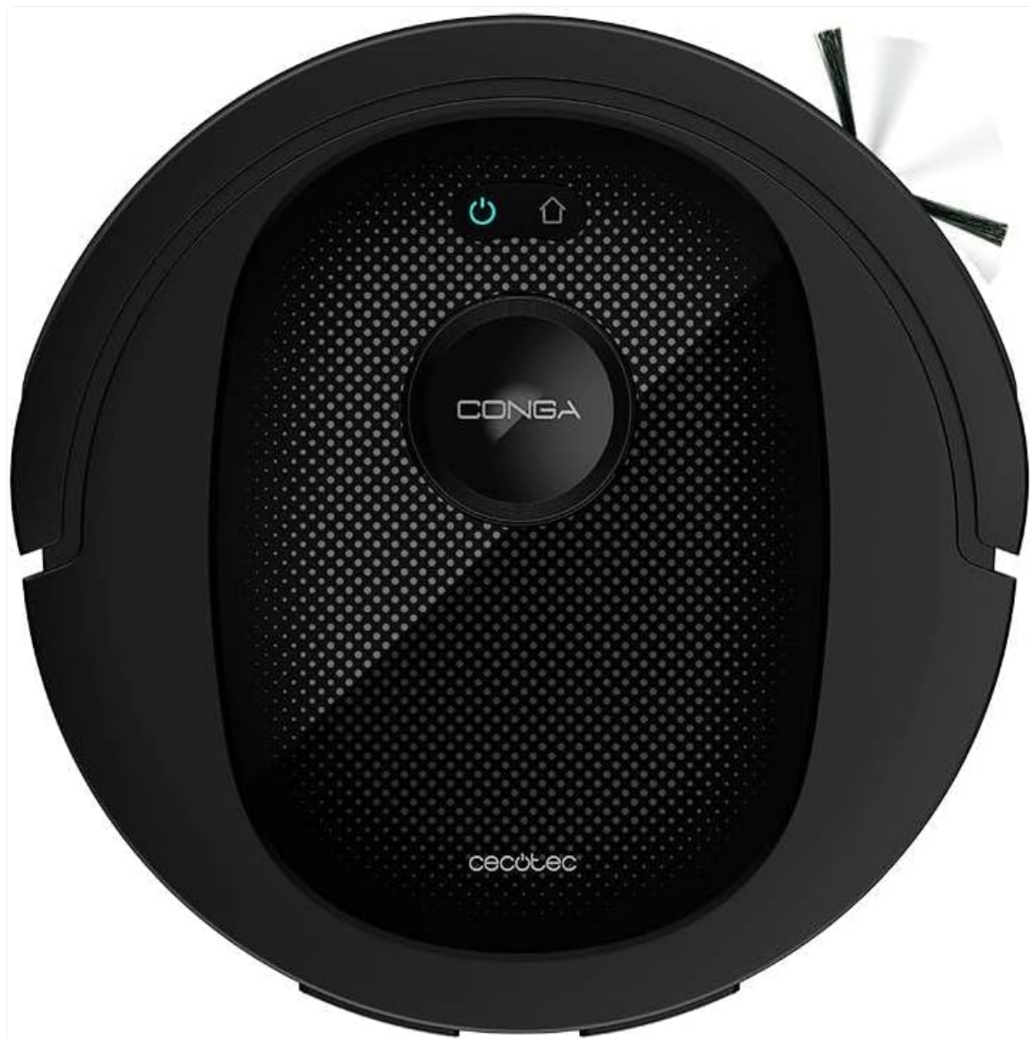
Figure 4.1: Top view of the robot vacuum cleaner, highlighting the power and home buttons.
