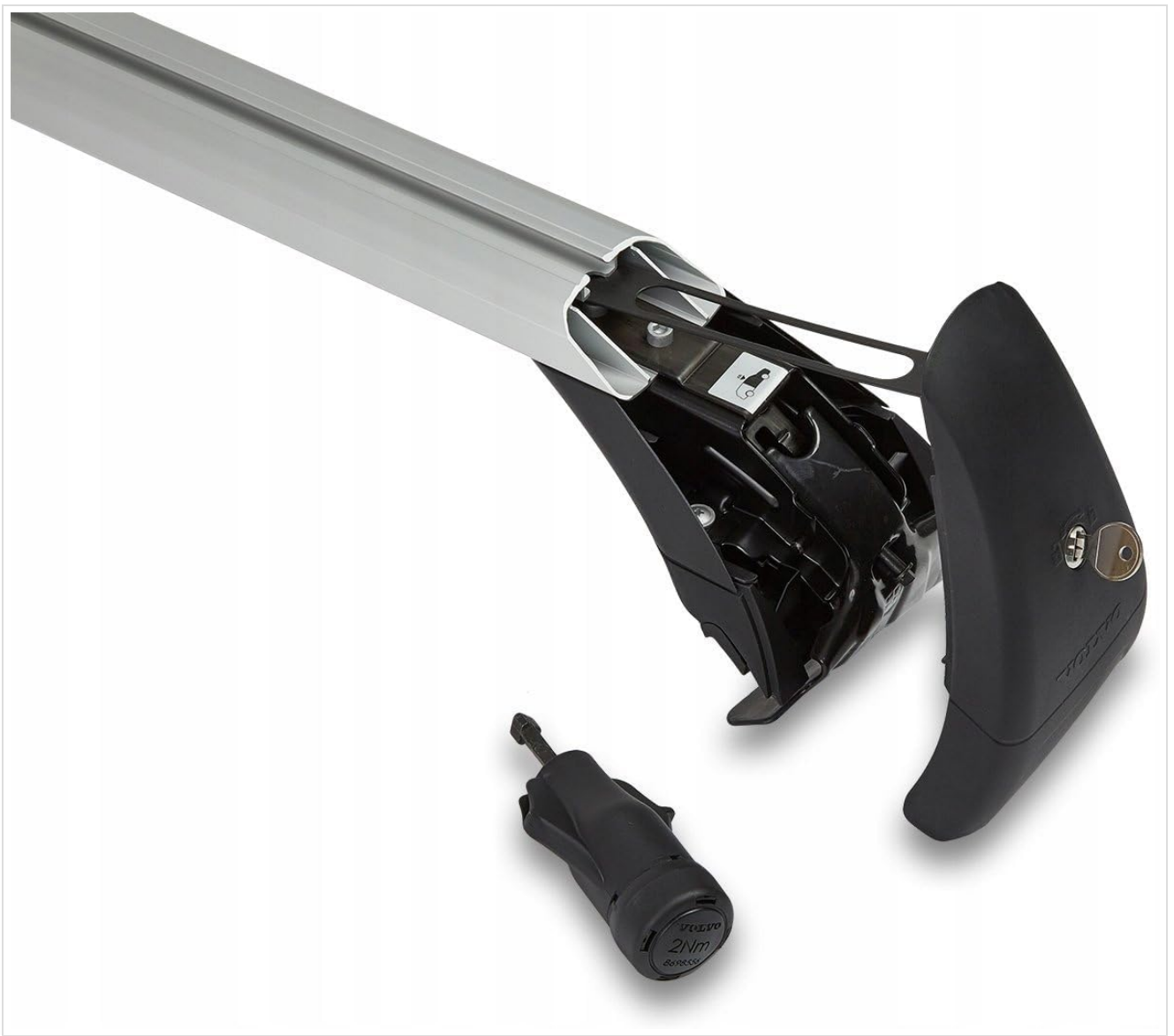
Figure 3: Detail of the roof rack's internal mechanism, showing a torque adjustment tool and a label indicating a 2Nm torque setting. This ensures proper tightening without overtightening.
