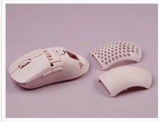
Image: The AJAZZ AJ199 mouse body with the solid back panel detached, showing the internal structure.
