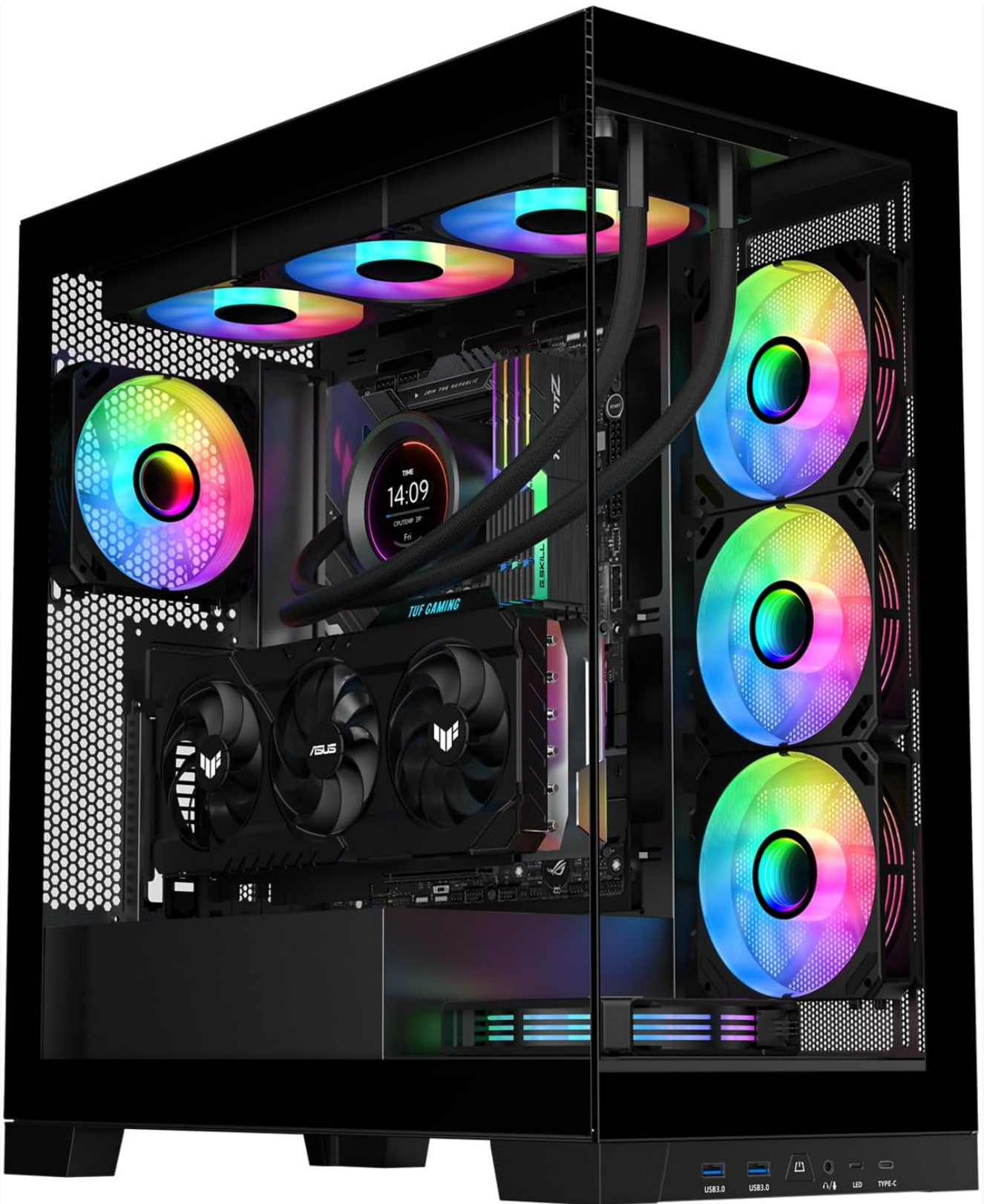
Image 1.1: SAMA NEVIEW 4503 Mid Tower PC Case, showcasing its dual tempered glass panels and pre-installed ARGB fans.
