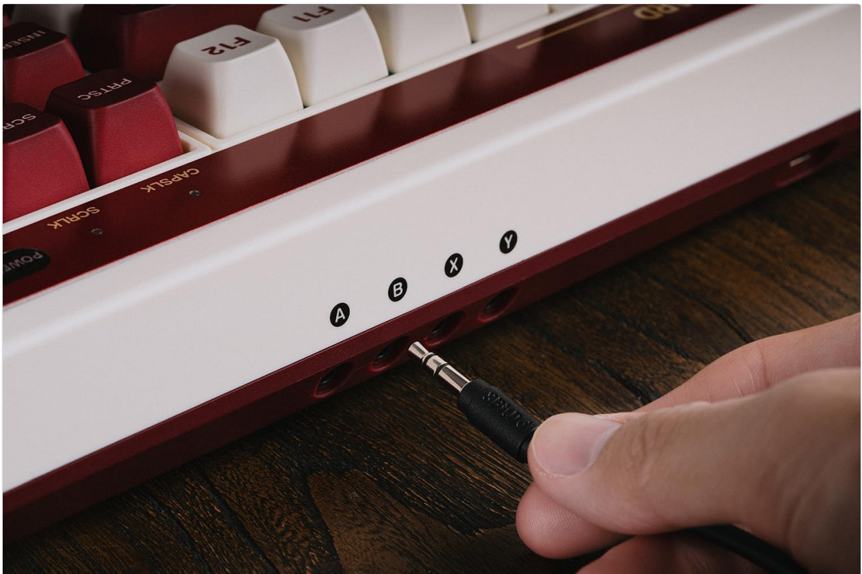
Image: A hand connecting the 3.5mm audio jack from the Dual Super Buttons into the corresponding port on the side of the keyboard.
