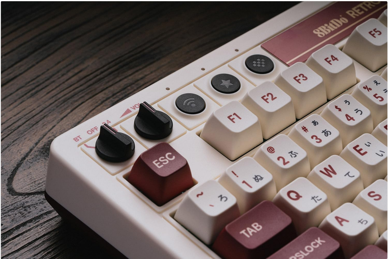
Image: A detailed view of the keyboard's independent control panel, showing the power switch, volume knobs, and connection mode selector.
