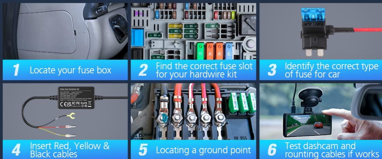
Figure 5: Visual guide for the hard-wire kit installation process within a vehicle.
