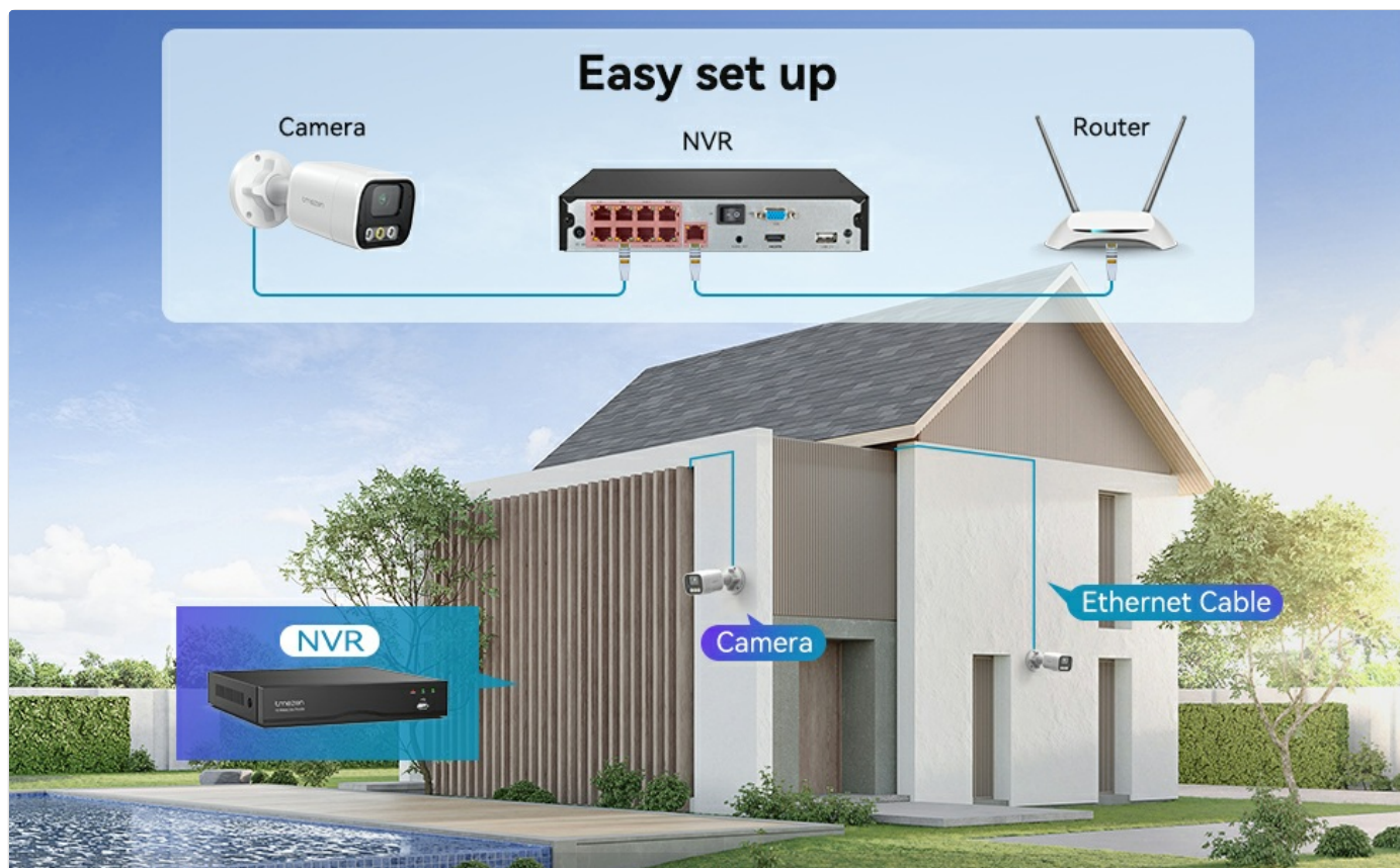
Image 4.1: Easy Setup Diagram. Shows how cameras connect to the NVR via Ethernet, and the NVR connects to a router for network access.
