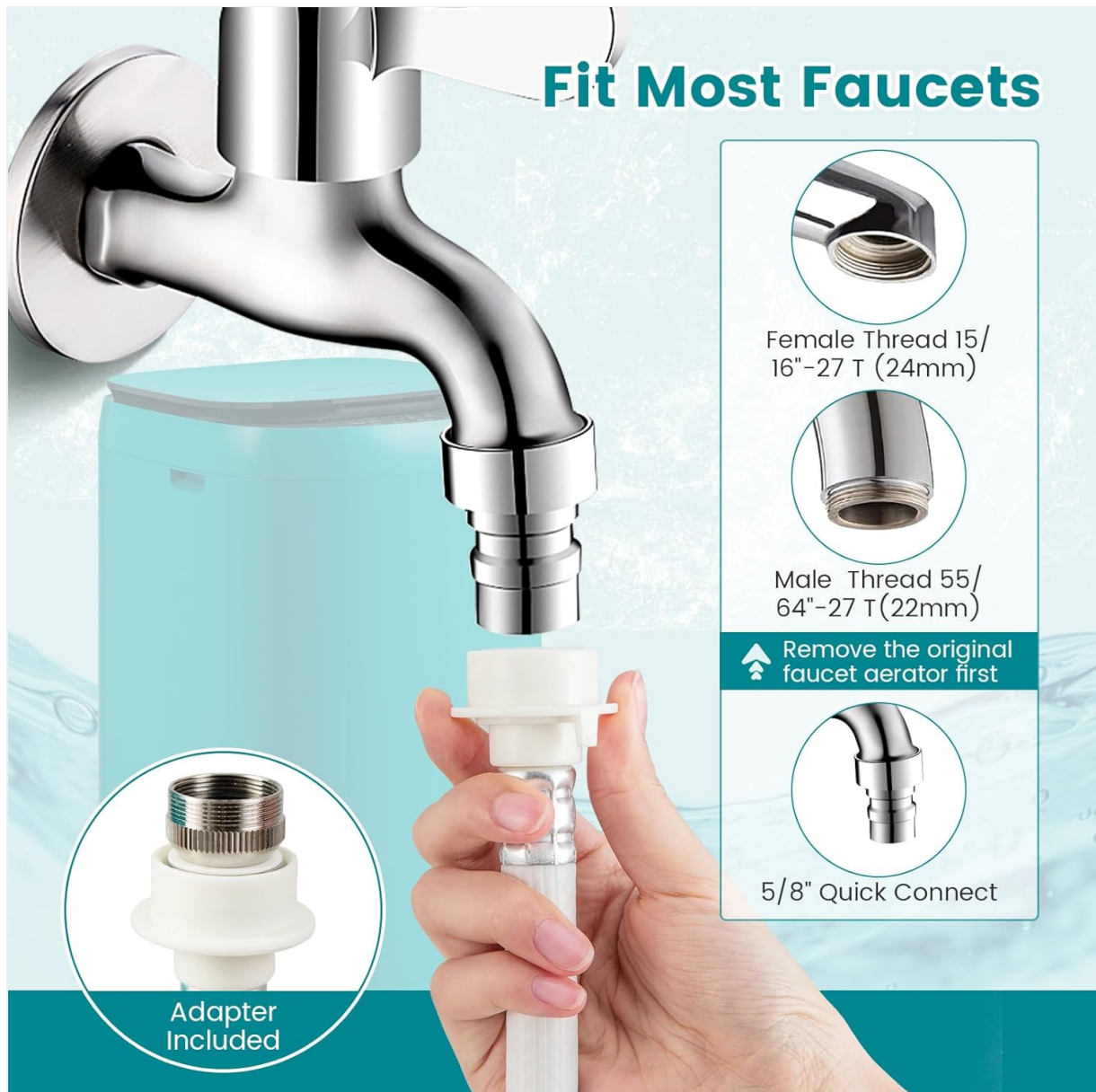
Image 3.2: This image demonstrates how to connect the inlet hose to a faucet using the provided adapter, highlighting compatible faucet thread types.
