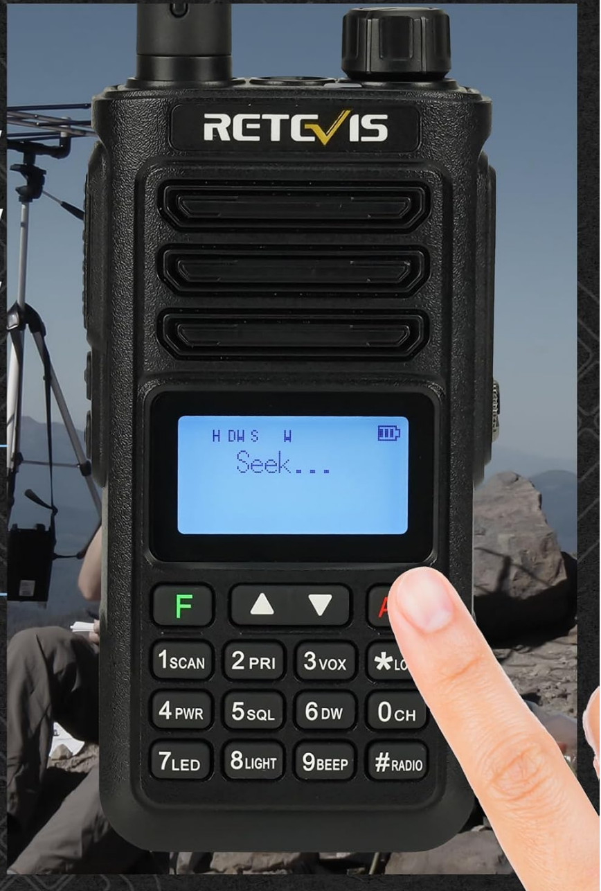
Figure 5.2.1: Using the A/B button for one-key frequency copy.
