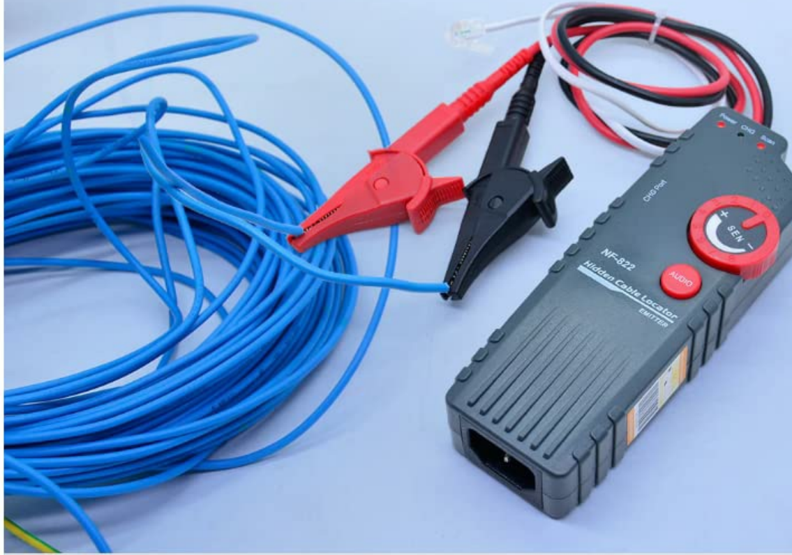
Image: The NF-822 transmitter connected to a bundle of blue cables, demonstrating a typical setup for tracing underground or hidden cables.
