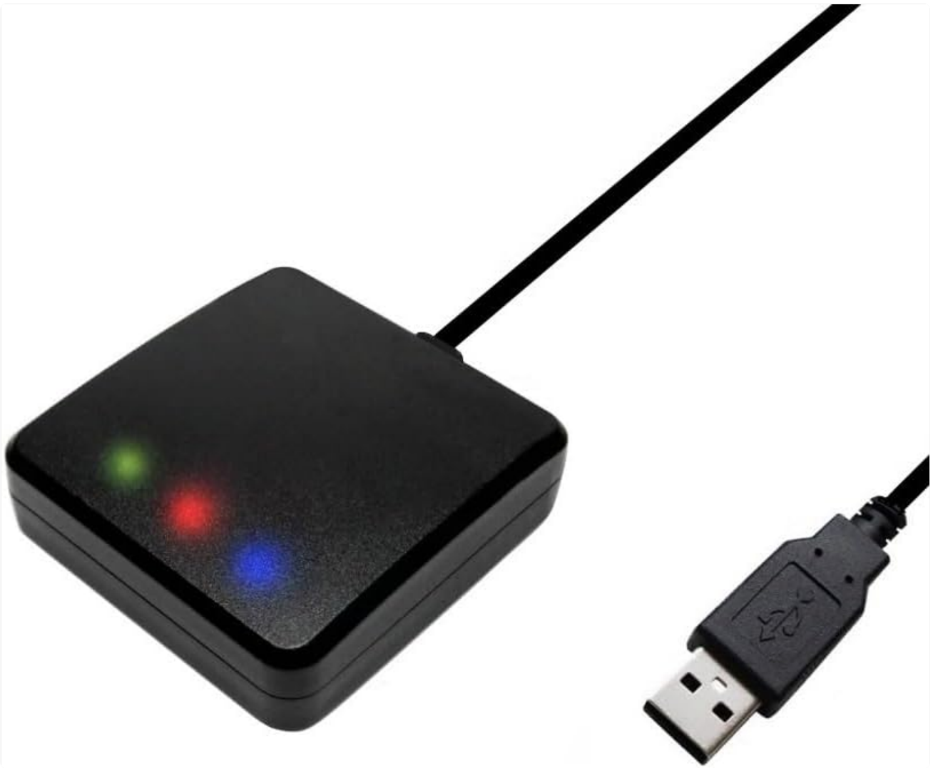
Figure 1: The LU23030-V2 GNSS receiver with its integrated USB cable. The device features indicator lights for status feedback.
