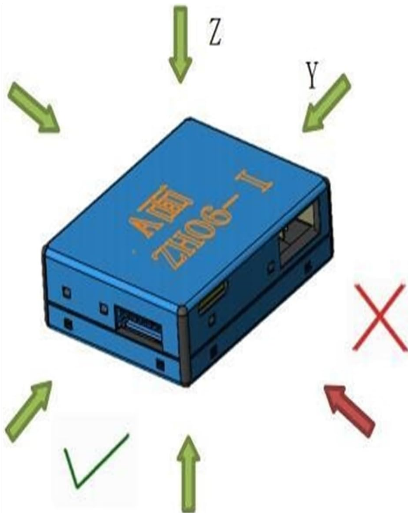
Figure 4: Optimal Airflow Direction (Green arrows indicate preferred directions, red X indicates undesirable direction)
