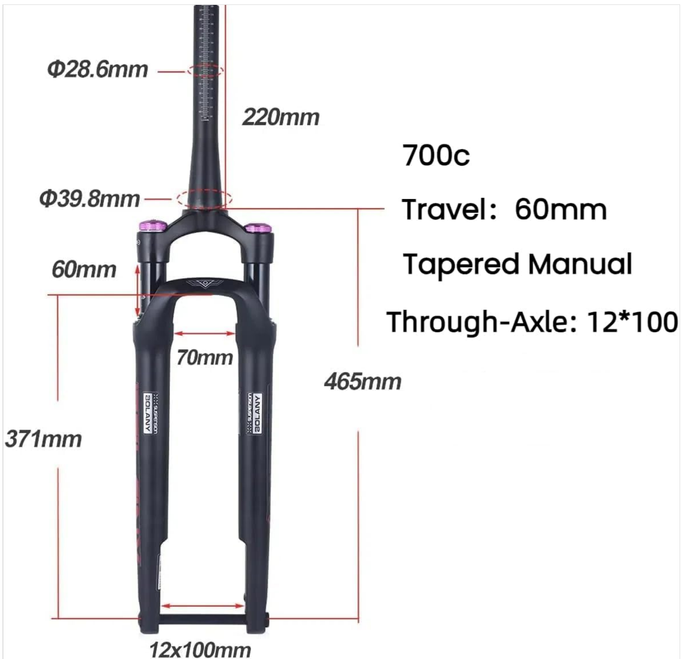
Figure 2: Key dimensions of the BOLANY 700C Air Suspension Fork. This image illustrates the steerer tube diameter (28.6mm and 39.8mm tapered), steerer tube length (220mm), travel (60mm), axle type (12x100mm), and overall fork length (465mm).
