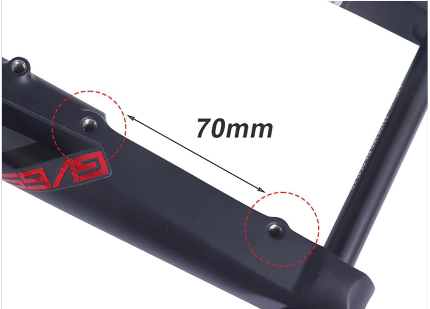
Figure 4: Detail of the International Standard A-pillar disc brake mount, indicating a 70mm spacing for caliper attachment. This mount is compatible with 160mm disc rotors.
