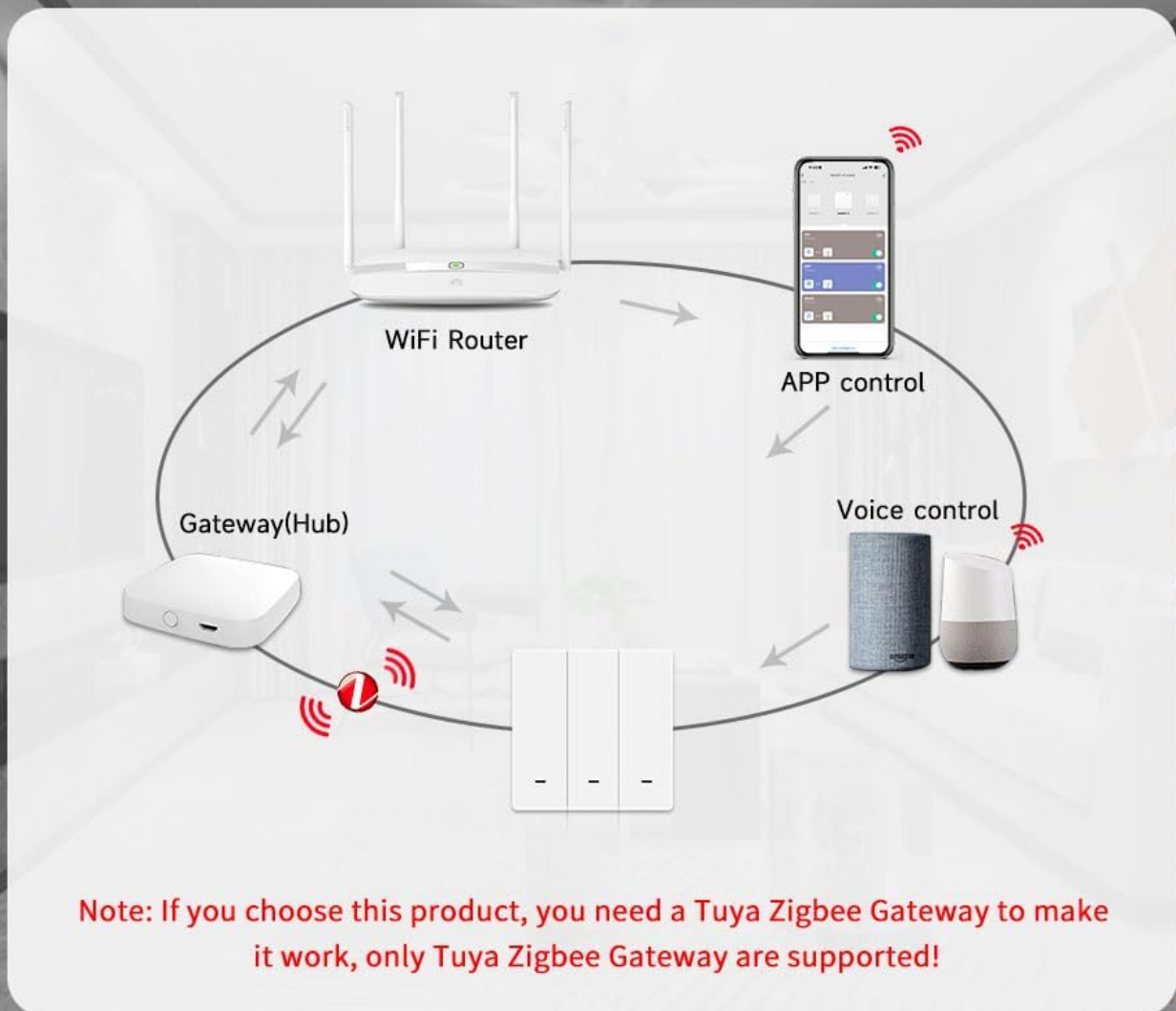
Image 2.1: Diagram illustrating the connection flow between the WiFi Router, ZigBee Gateway (Hub), mobile APP control, voice control, and the Smart Scene Switch.
