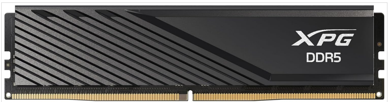
Image 2.1: Top view of an XPG Lancer Blade DDR5 RAM module. Note the notch on the gold contacts for correct alignment with the motherboard slot.
