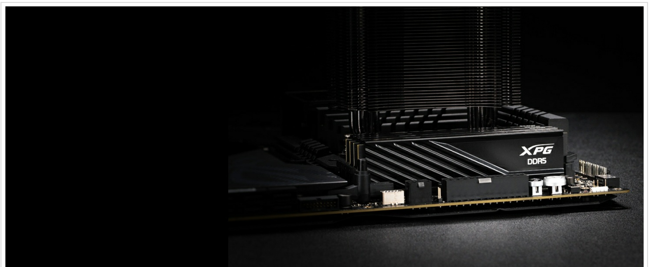
Image 4.1: XPG Lancer Blade DDR5 memory with a low-profile heatsink. This design ensures compatibility with various CPU coolers and improves thermal performance.
