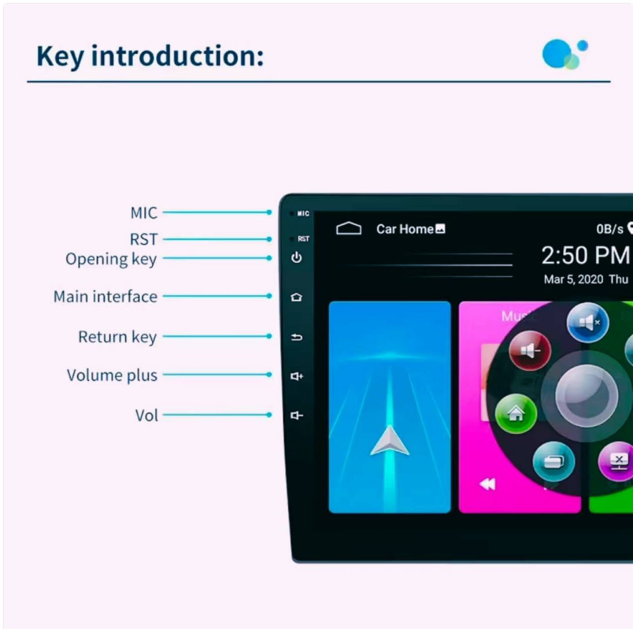
Figure 4.1: Front Panel Key Introduction. This diagram illustrates the functions of the buttons and ports on the front panel of the car stereo, including Microphone, Reset, Power/Opening Key, Main Interface, Return Key, Volume Up, and Volume Down.
