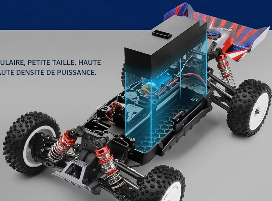
Image 5.1: Installing the modular battery into the RC car.
