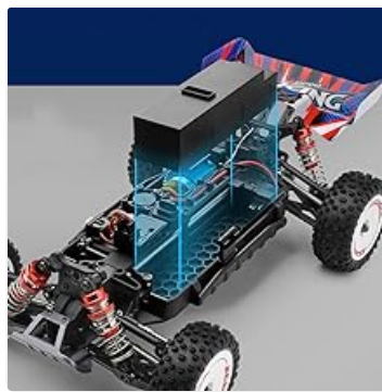
Image 4.1: Internal view of the RC car chassis, showing the brushless motor and battery compartment.
