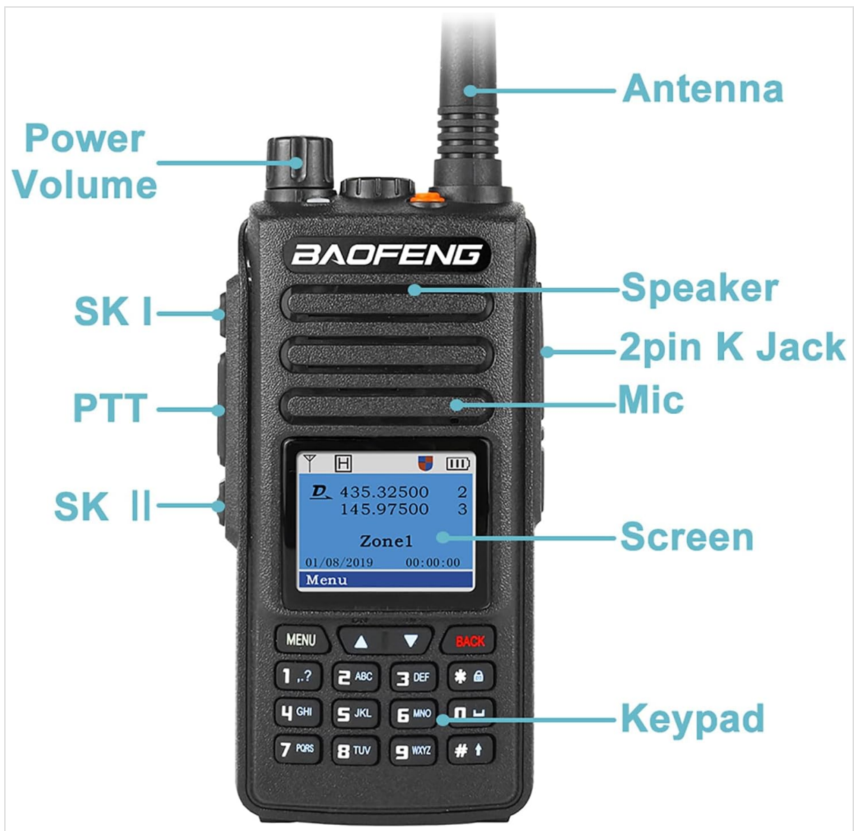
Figure 9.1: Dimensions of the BAOFENG DM-1702 Radio.
