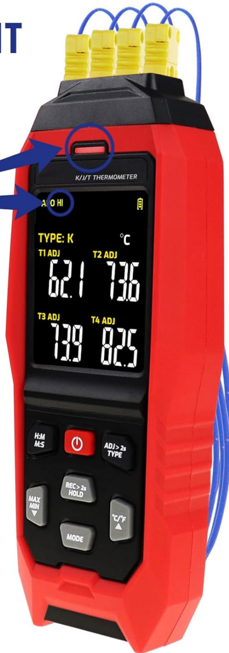
Image: The thermometer's display showing the wide temperature range capabilities for K, J, and T-type thermocouples, alongside four K-type probes.
