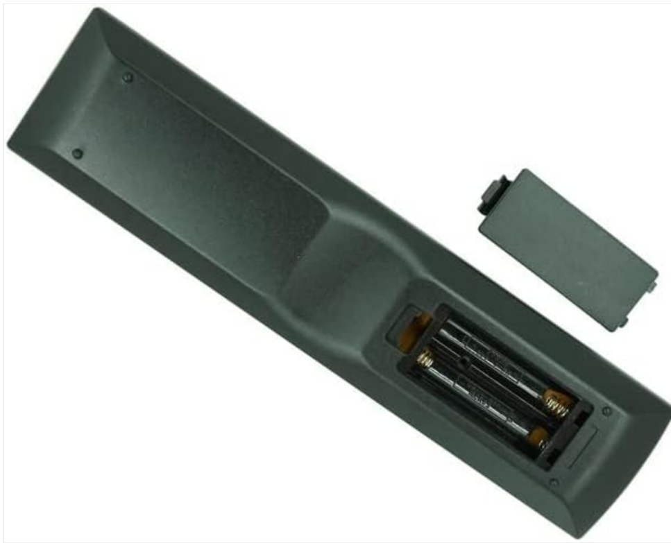
Figure 2: Back of the remote control with the battery compartment open, illustrating the correct battery placement.
