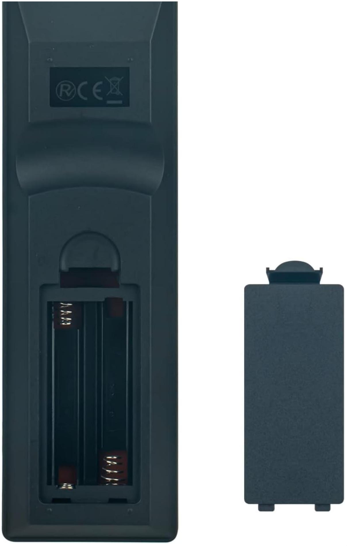
Figure 1: Battery compartment of the R230D1A remote control. Insert two AAA batteries according to polarity markings.
