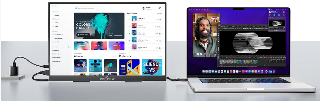
Image: Illustrations demonstrating how to connect the monitor to a laptop using a single USB-C cable for power and video, and using an HDMI cable with a separate power cable.
