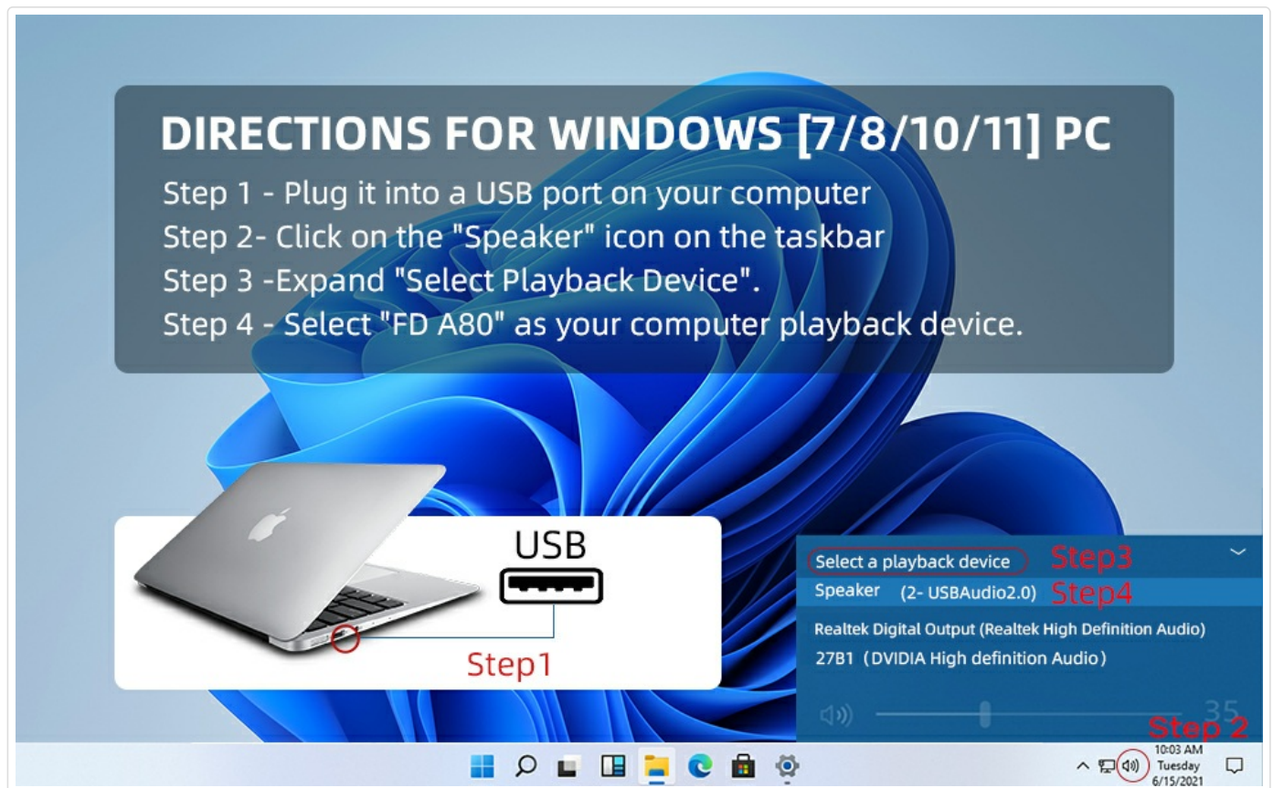
Figure 5.2: Visual guide for setting up the HEANTTV A80 soundbar on Windows 7/8/10/11 PCs, showing the steps to select 'FD A80' as the playback device from the taskbar speaker icon.
