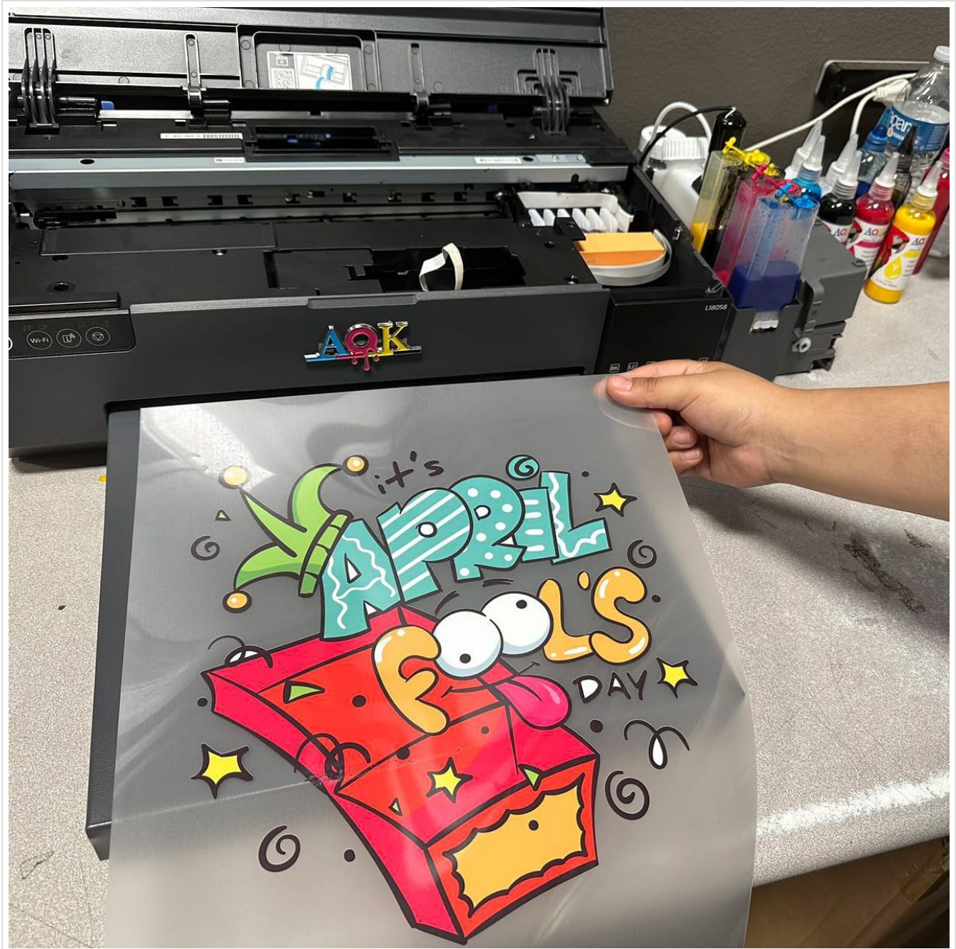
Image 5.1: A printed DTF film showing a colorful design, ready for powder application and curing.
