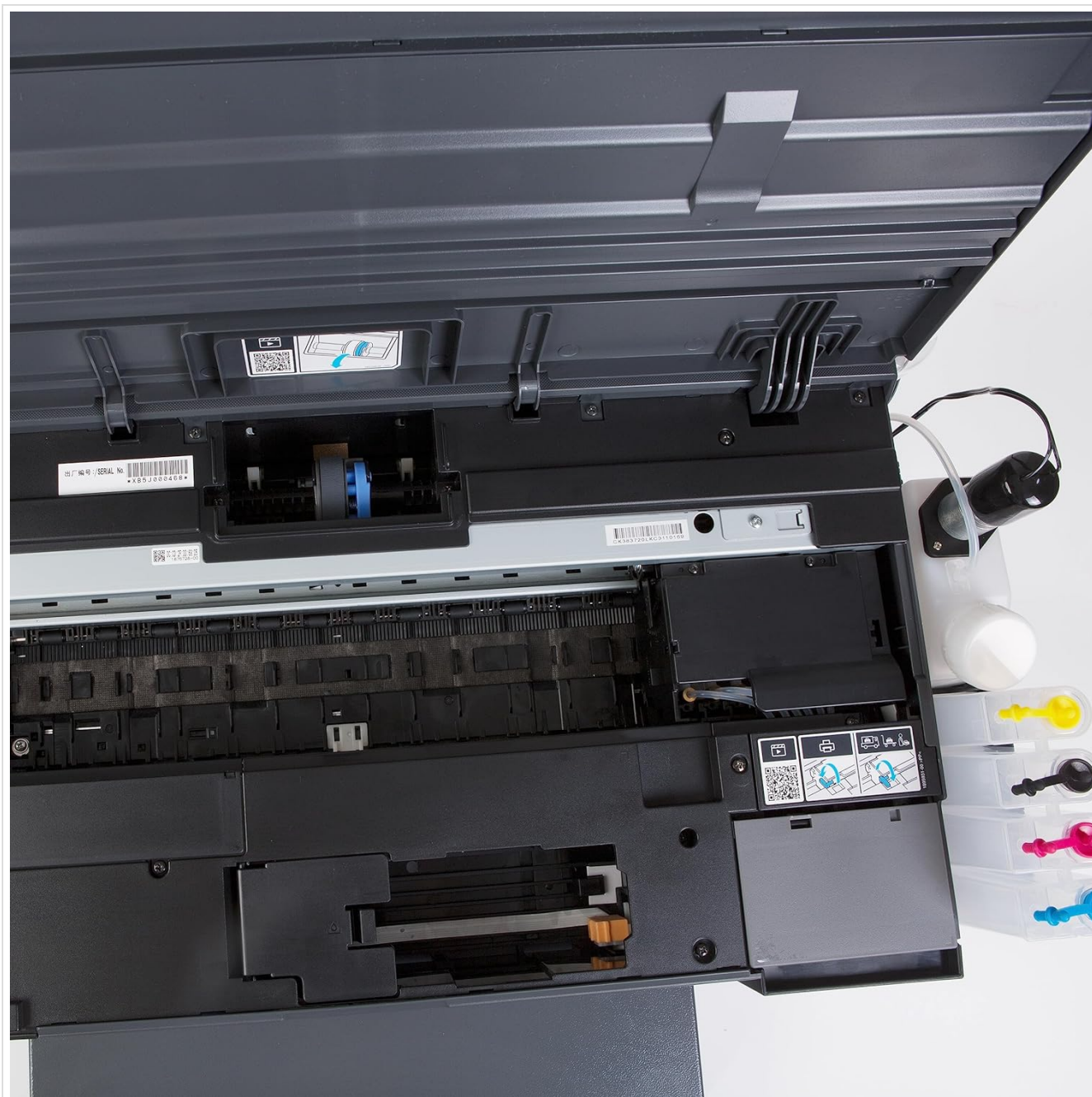
Image 6.1: Internal view of the printer, highlighting the printhead and ink delivery system, critical areas for maintenance.
