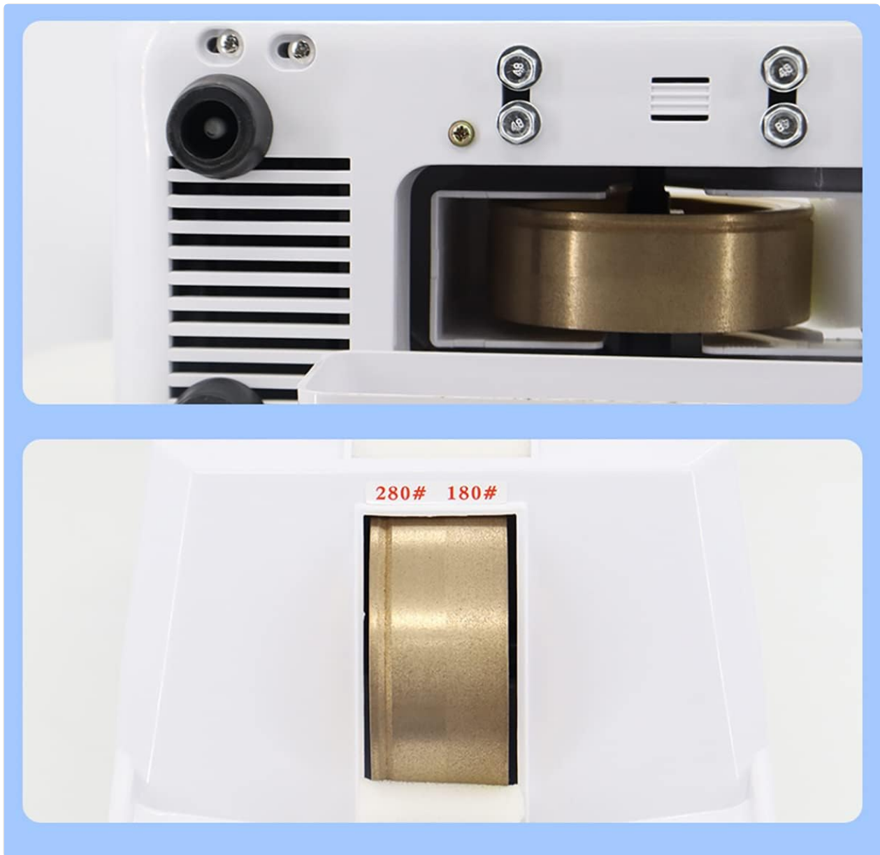
Figure 5.2: Top-down view of the grinding wheel, indicating the grit sizes for different stages of lens processing.
