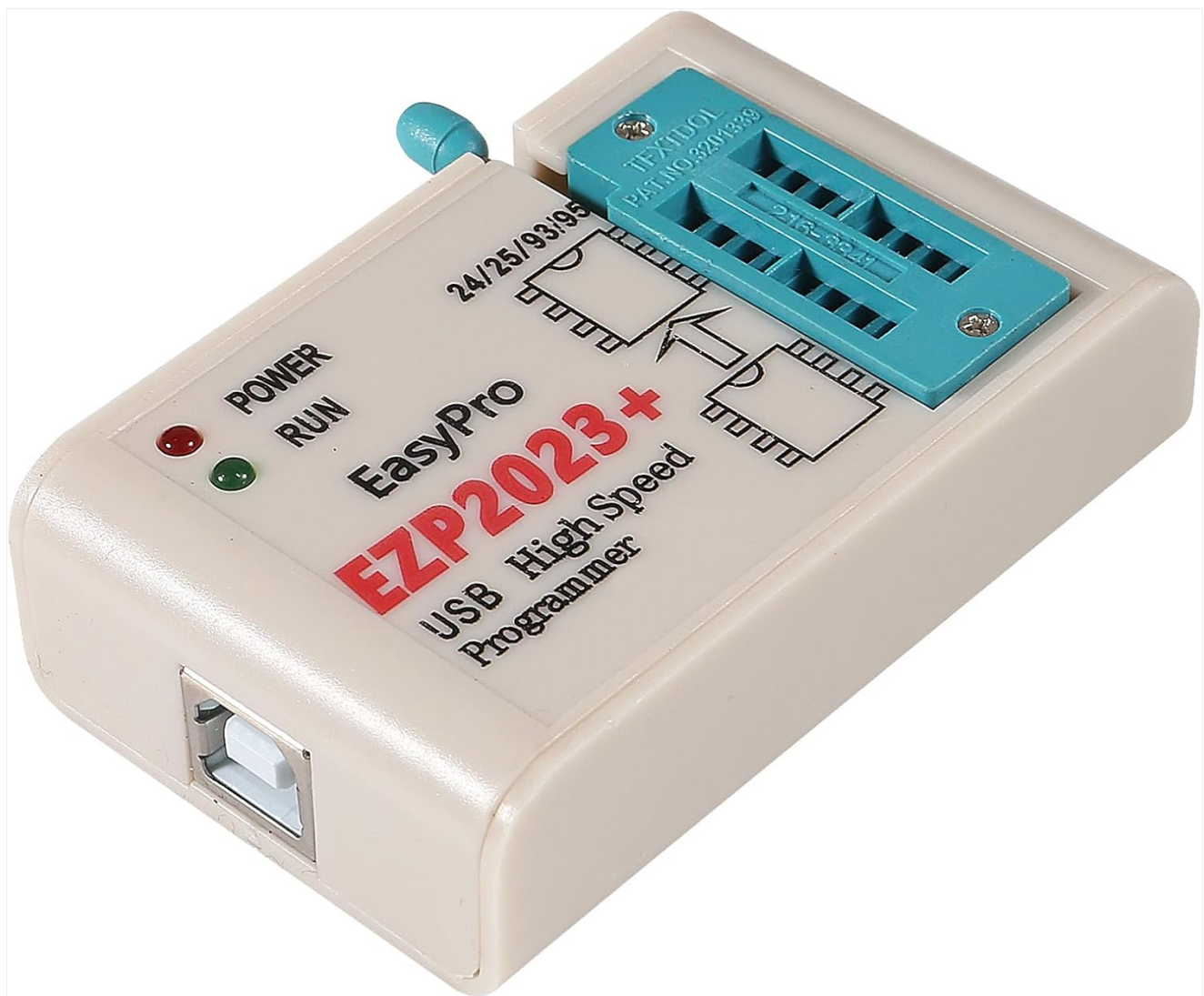
Figure 3: Detail view of the EZP2023 programmer, highlighting the USB port for connection to a computer and the ZIF socket for chip insertion.
