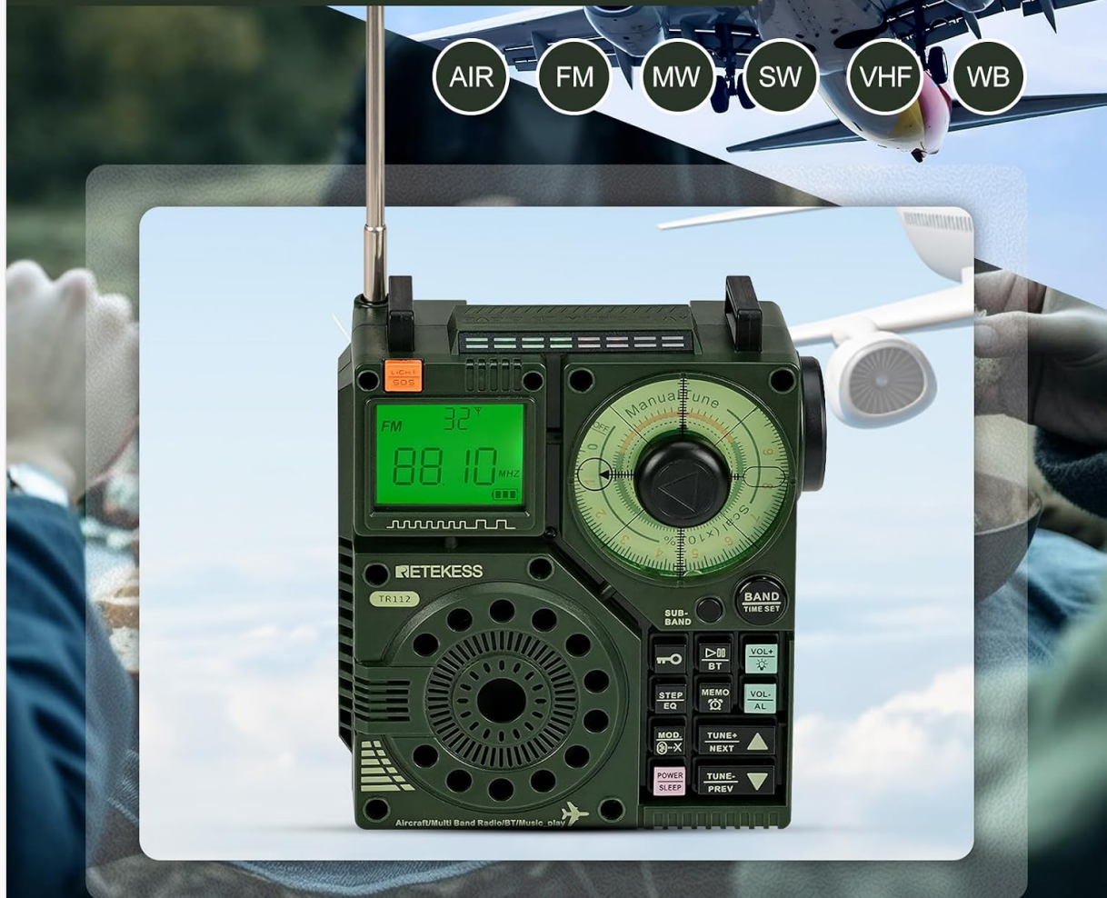
Figure 5.1: Supported frequency bands of the TR112.
