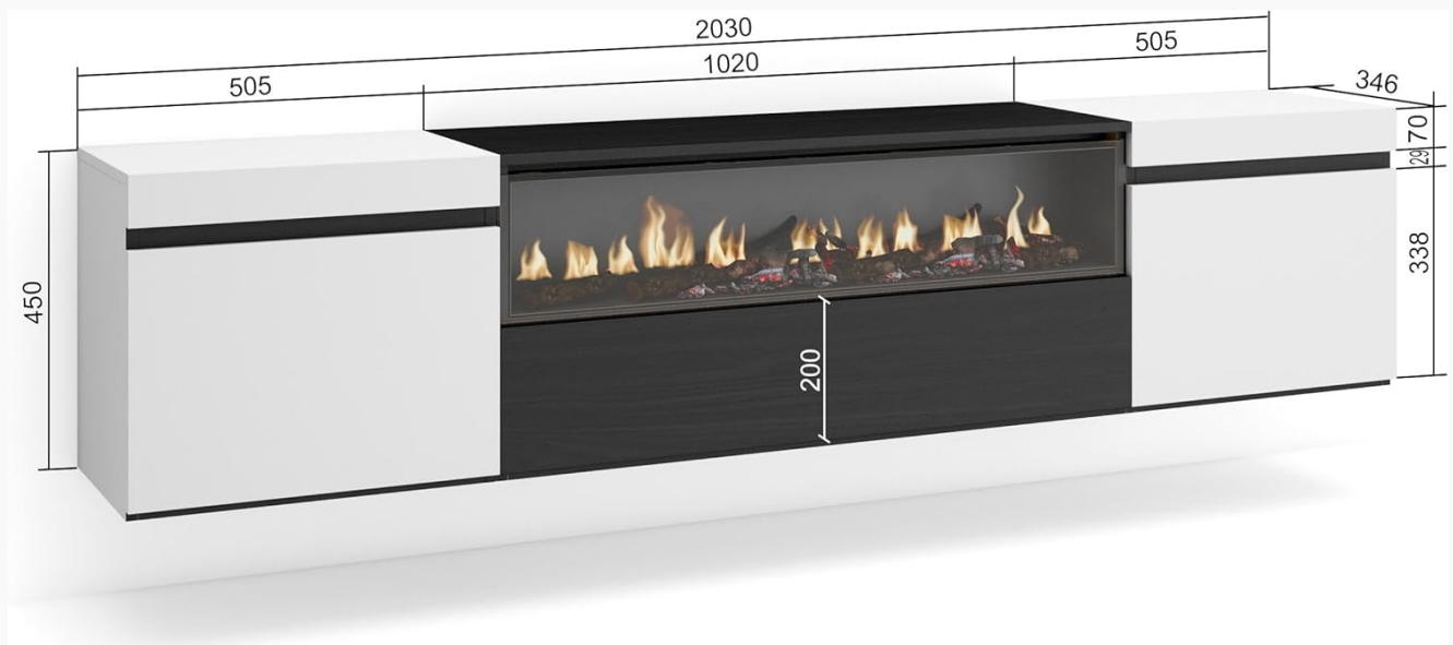
Image: A technical diagram illustrating the overall dimensions of the TV cabinet, including the 2030mm total width and individual module widths (505mm for side modules, 1020mm for the central module).
