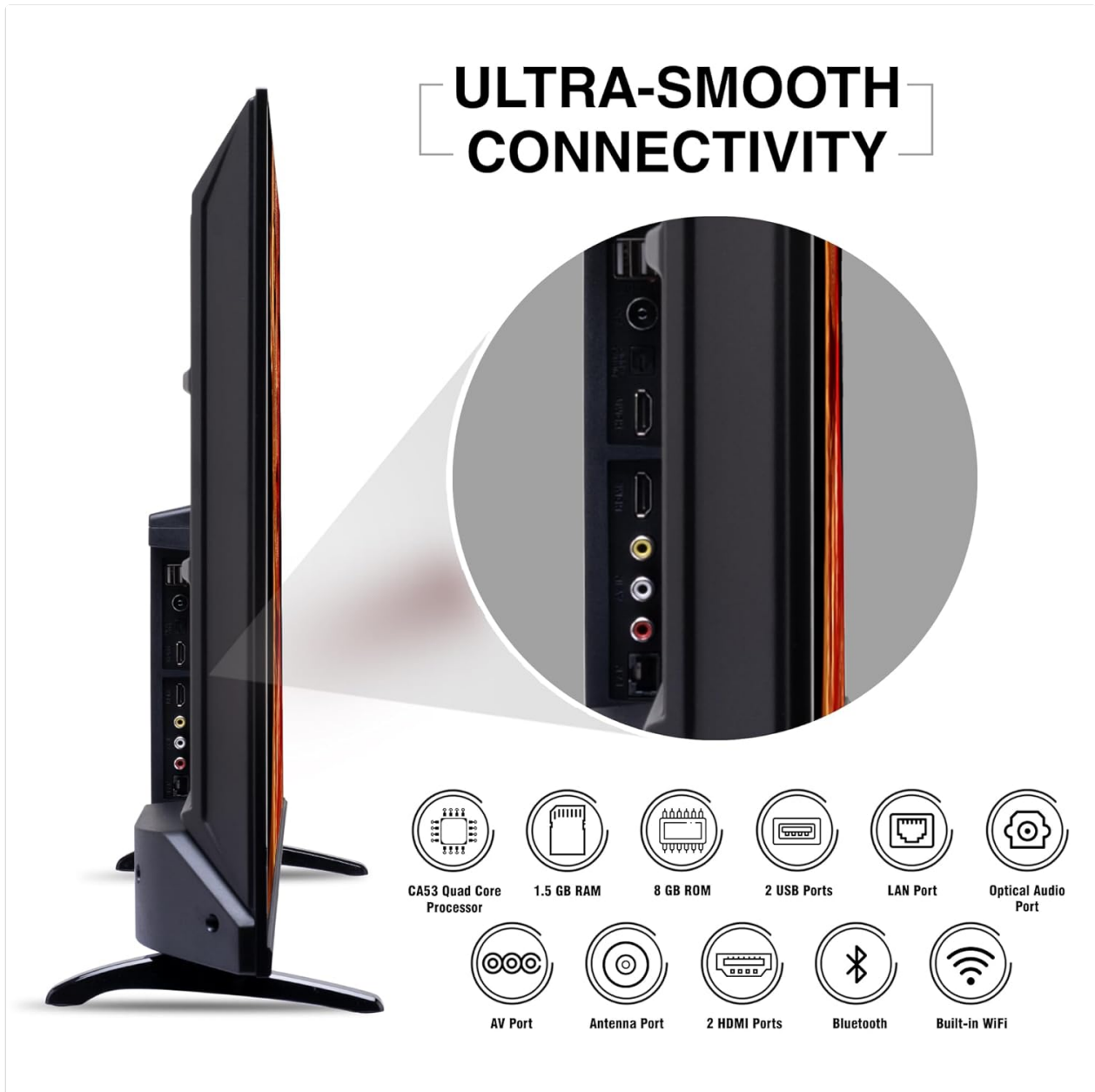
Image 4.2: Side view of the SANSUI TV highlighting various input/output ports.
