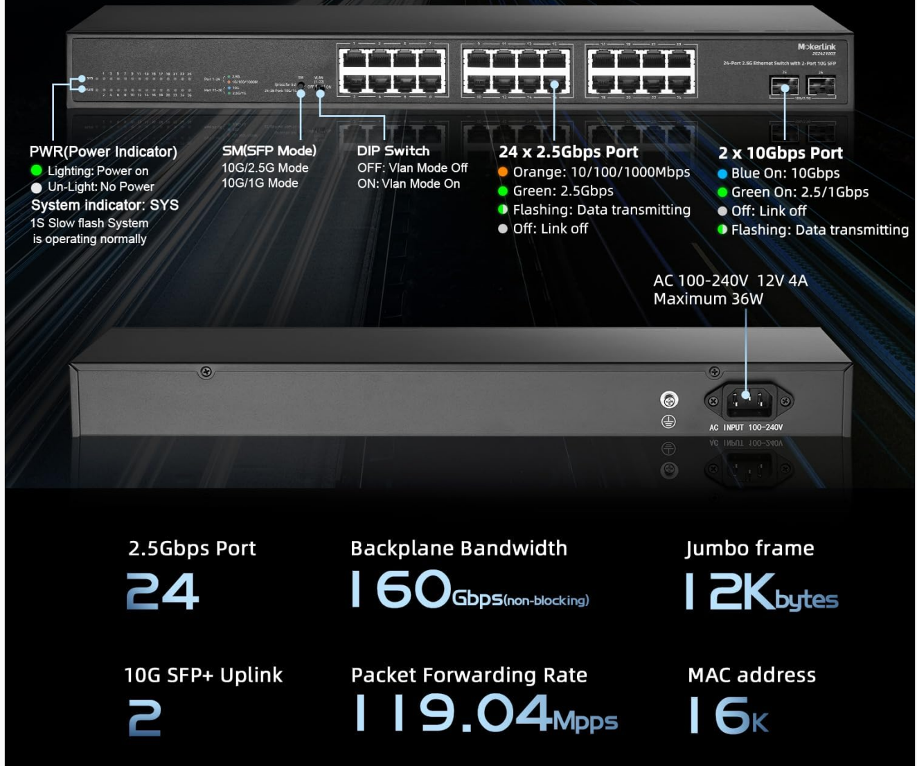
Image 2.2: Detailed port configuration, LED indicators, and power input on the switch.
