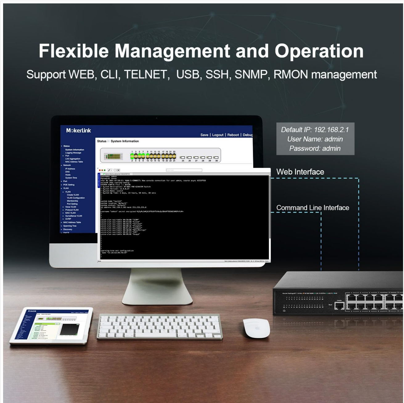
Figure 5.1: Web and Command Line Interfaces for switch management.
