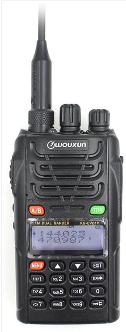
Image Description: A front view of the Wouxun KG-UVD1P FM Transceiver, showcasing its black casing, antenna, LCD display, keypad, and control knobs. The display shows frequency information.
