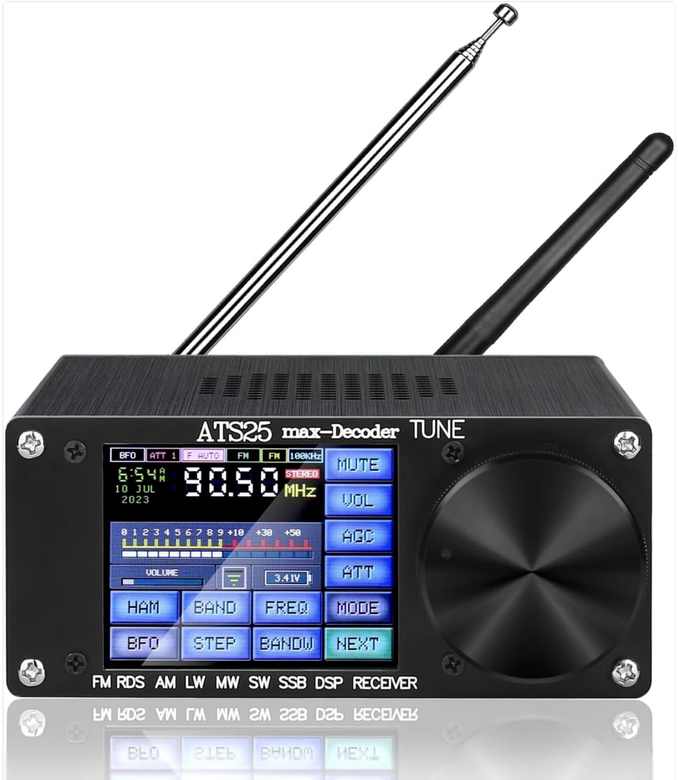
Figure 1: Front view of the ATS-25 max-Decoder radio receiver. This image highlights the main display, tuning knob, and control buttons for functions like HAM, BAND, FREQ, MODE, BFO, STEP, BANDW, and NEXT. Both a telescopic and a stubby antenna are shown attached.
