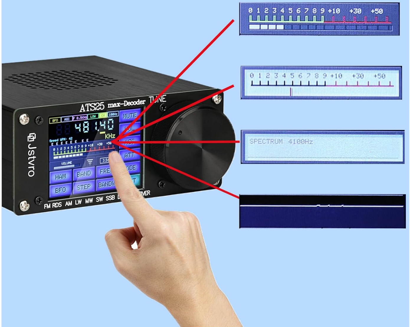
Figure 6: CW Network Signal Formats. This image demonstrates the radio's ability to display CW signals in various visual formats, with instructions to use a stylus to change the format.
