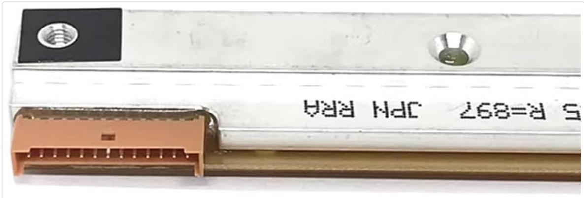
Figure 4: Close-up of one of the printhead's electrical connectors, showing the pin configuration for proper connection.
