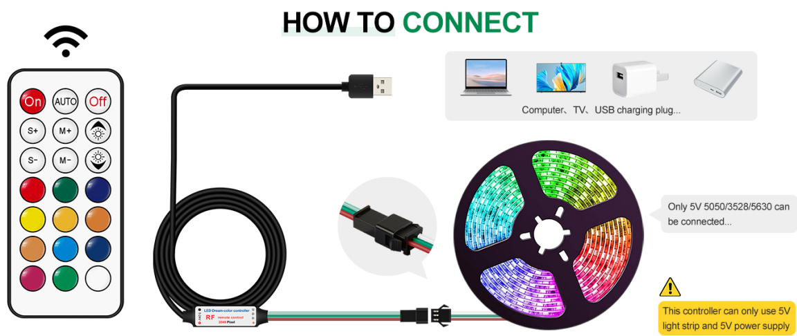
Image 3.1: Connection diagram for the LED controller, power adapter, and LED strip.
