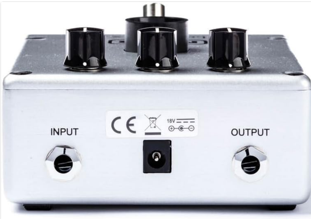
Figure 3: Rear view of the MXR M222 Talk Box, showing the input, power, and output connections.
