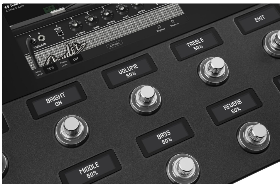
Image: Detailed view of the footswitches and their corresponding LCD scribble strips, showing various effect parameters.
