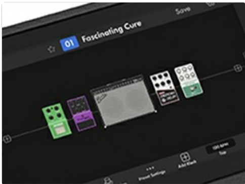
Image: A digital representation of a guitar signal chain on the Tone Master Pro's screen, illustrating how effects and amps are connected.
